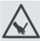
Beware. After turning the verticutter off, the blade keeps rotating for a while!
